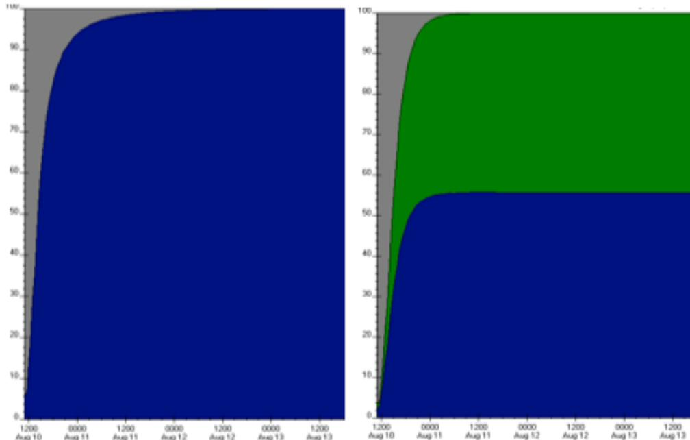
ADIOS2 model output for a jet fuel spill of 100 bbl, winds of 5 knots (left) and 7 knots (right). Blue = evaporated; green = dispersed; grey = remaining. Jet fuel and kerosene are lighter than diesel/No. 2 fuel oil, with higher rates of evaporation under similar conditions.
