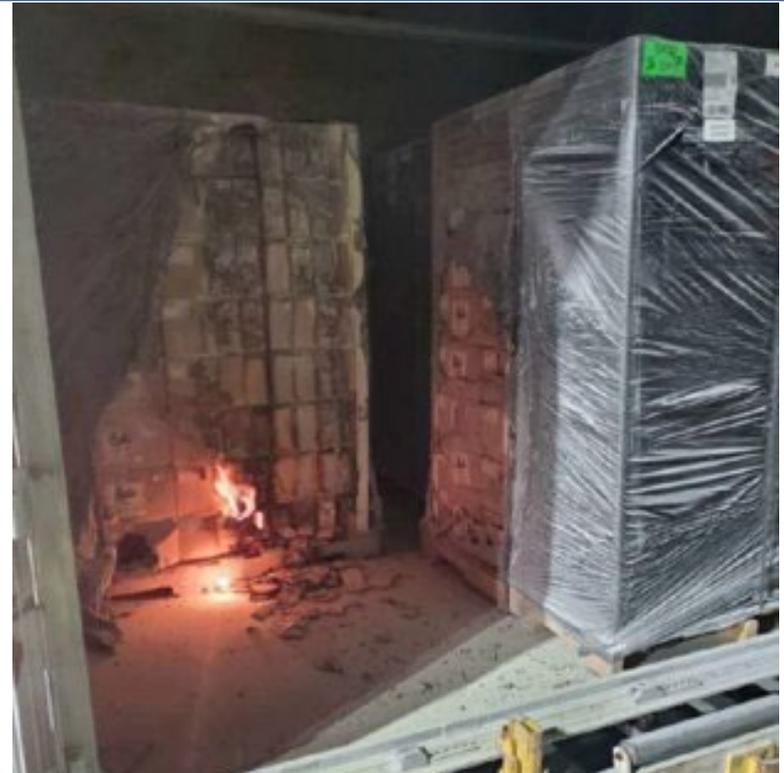
Use of black shrink-wrap made it difficult to see damage that impacted the cellphones/batteries in the packages.
