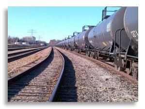
Rail shipments of petroleum crude oil typically consist of unit trains of over 100 tank cars, with each tank car containing approximately 30,000 gallons of crude oil.
