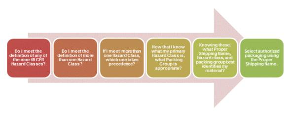
The HMR provides a safety system that, when implemented properly, can help prevent transportation incidents, mitigate the consequences of such incidents should one occur, and communicate the hazards and emergency response information. The effectiveness of this safety approach is, in part, dependent on the proper classification and characterization of the hazardous material being transported. The improper classification and/or characterization can diminish the intended effectiveness of the HMR.
