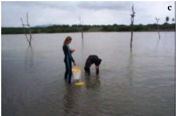
Figure 7. Mouth of Boac River: a) Detail of the river mouth meeting the ocean; b) Dr. Carr taking GPS coordinates at sampling station 9 and Marinduque field team on the river's edge helping with sampling gear; c) Drs. Carr and Nipper collecting sediment for porewater extraction.
