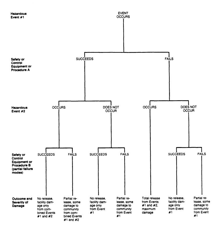
unwanted event, such as a release of toxic materials, could possibly occur. The technique, which in structure is similar to the event analysis technique, involves the development of fault tree diagrams which illustrate the "chain of events" required for a particular event to occur.
