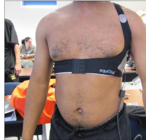
The Sensor Electronics Module (SEM) is hardwired to a cell phone which was attached to the arm or a waist belt
